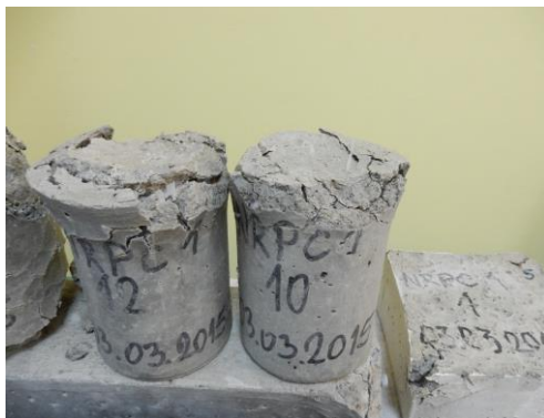
Figure 10-Appearance of samples exposed to \text{Na}_2\text{SO}_4
