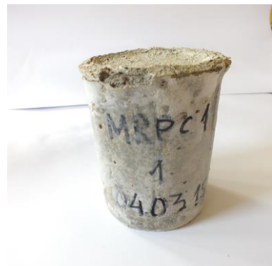
Figure 11-Appearance of samples exposed to \text{MgSO}_4
