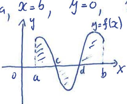
$$P = \int_a^c f(x) dx - \int_c^d f(x) dx + \int_d^b f(x) dx$$
